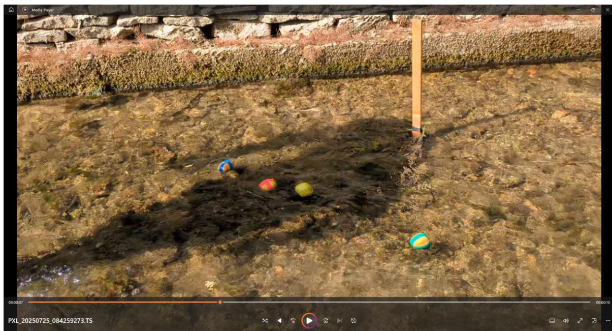
Figure 5 Example Frame from Shortly After a Cluster of Apples Were Released from a Central Subsection of the Stream. Some Longitudinal and Lateral Dispersion is Already Evident only a Few Seconds after Release.
